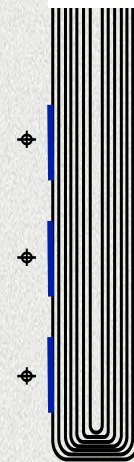
AEGIS recommendation: 22' loose tube with three 3' targeted sections of laser clad using higher hardness material
